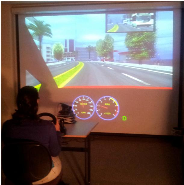
**Fig. 1.** The experiment setup. The participant is sitting in a clerical chair, holding the wheel, while the scenario is presented on a wide screen in front of her.
