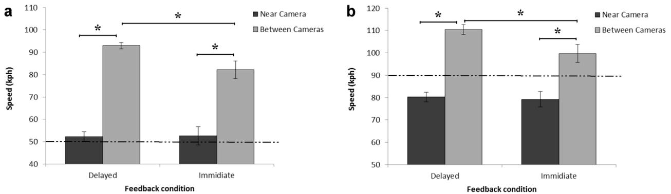
**Fig. 10.** Median speed as function of camera proximity and feedback condition: (a) speed limit = 50 kph; (b) speed limit = 90 kph. \*\*\* denotes simple comparisons significant differences. The dashed line represents the speed limit. The error bars reflect standard errors.
