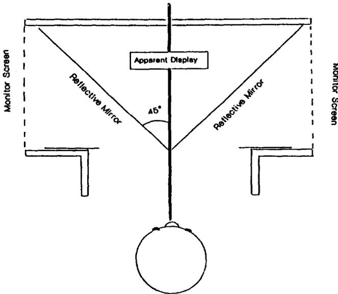
Fig. 1. Schematic top view of the optical arrangement used.
