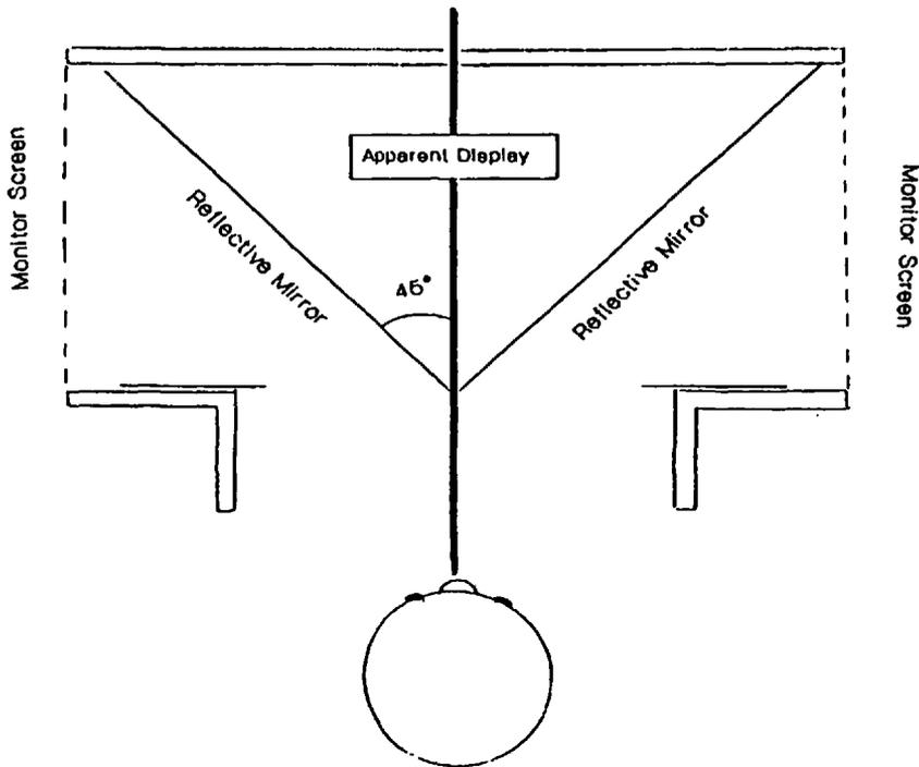
Figure 2. Schematic top view of the optical arrangement used. There was no partition in the binocular viewing condition.
