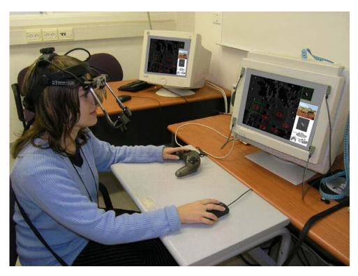
Figure 8. A participant sitting opposite the screen with an eye-movement monitor on her head and a second computer in the background for gathering the eye-movement data
