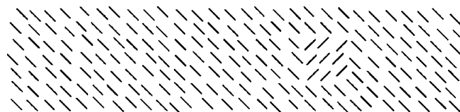
Fig. 1. A schematic example of the texture displays used in Experiments 1 and 2. The texture line elements are oriented \pm 45^\circ from vertical and the texture display extends along the horizontal meridian. A 3 \times 3 target patch is visible in the display on the right.
